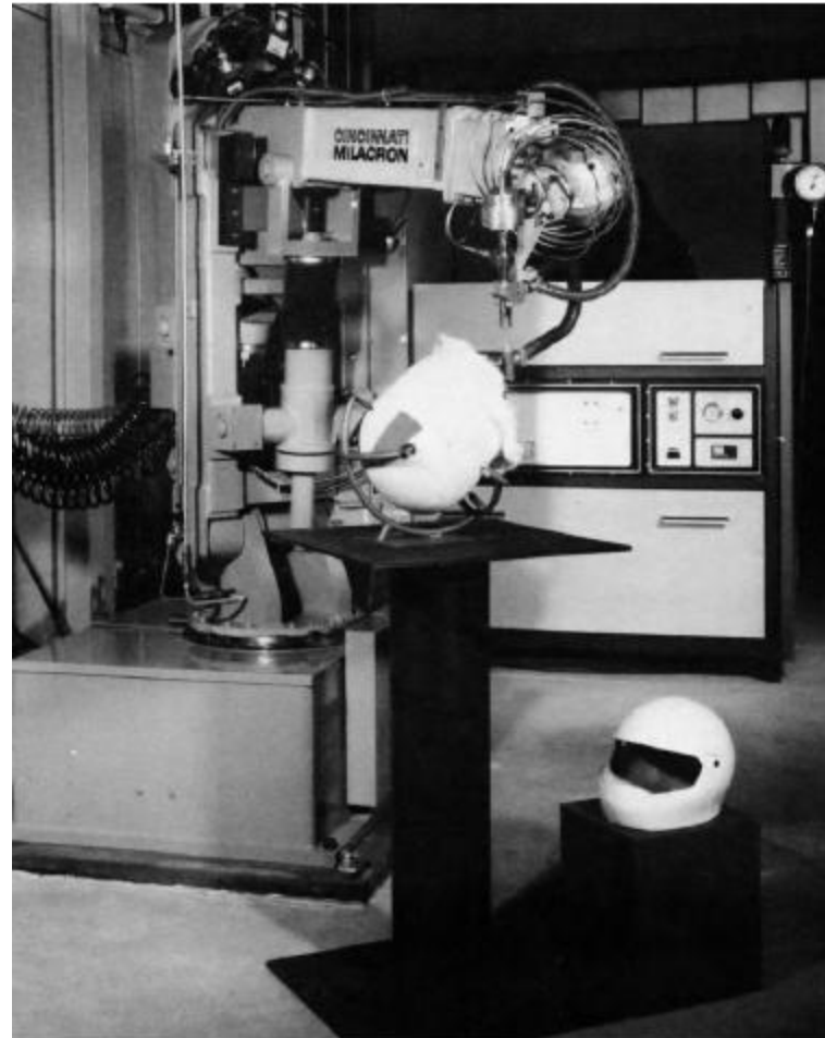
Figure 7.13 Cutting to shape of glass reinforced plastic crash helmets with a high pressure (3000 bar, 50,000 psi) water jet. The process produces a clean surface without creating injurious dust (courtesy of Cincinnati Milacron).
