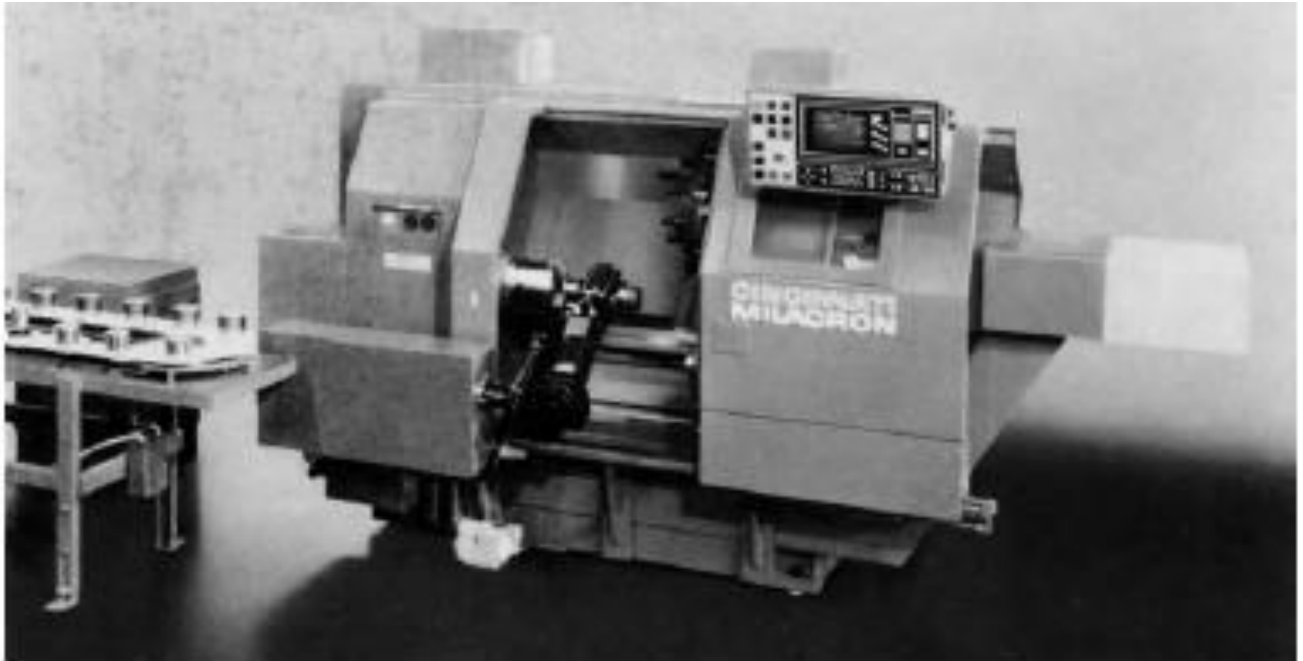
Figure 7.3 A numerically controlled lathe with a built-in loading robot (courtesy of Cincinnati Milacron).
