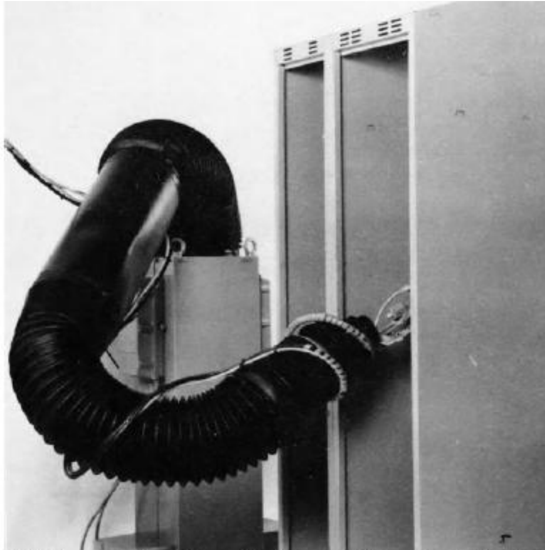
Figure 7.10 Paint spraying by a Spine robot: (a) a van interior; (b) a steel cabinet (courtesy Spine Robotics).
